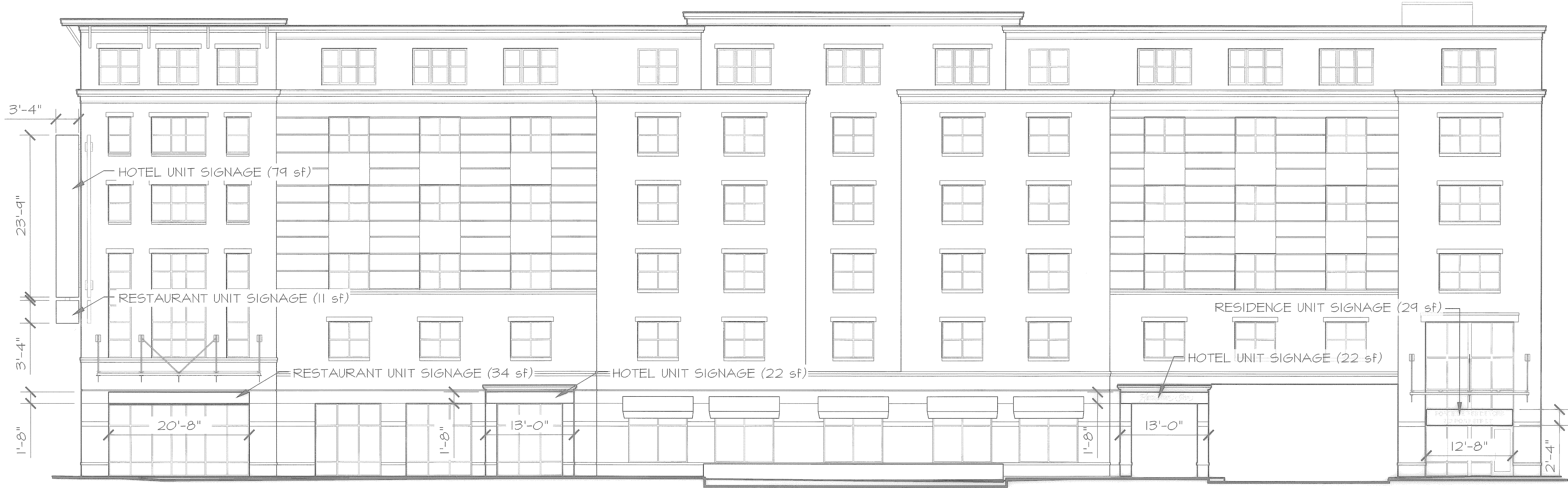
SOUTHEAST EXTERIOR BUILDING ELEVATION 1" = 8'-0"
